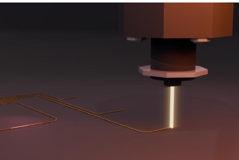
DALP is a non-contact, digitally controlled process, allowing for spatially resolved surface treatment with high precision. Unlike traditional post-processing methods, it does not require masks or physical contact, which reduces the risk of contamination and mechanical damage.
